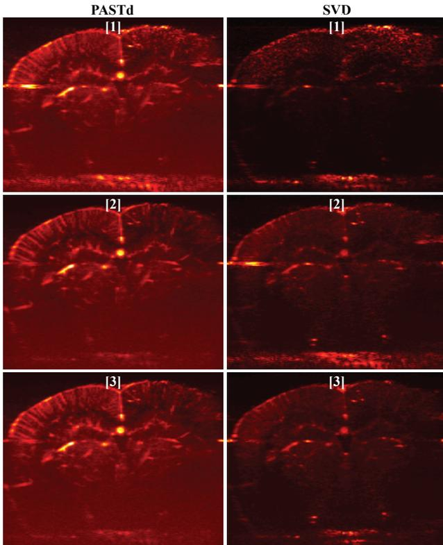
**Figure 2: Comparing the exponentially weighted PASTd method and the SVD method by sequentially removing eigencomponents.** The white number displays the number of removed components for each of the methods. It is clear that the exponential weighting of the PASTd method ( $\beta = 0.5$ ) greatly reduces the number of components needed to remove.
